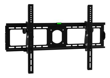
Tiltable LCD / TFT TV Wall Mount Material: 2.0mm Cold Rolled Steel Plate TV Size: 32" - 60" Tilt: 0 / +15 degrees Maximum load capacity: 165 lbs / 75 kgs Wall distance: 3.3" / 84mm Bubble level included Universal Mounting Pattern
